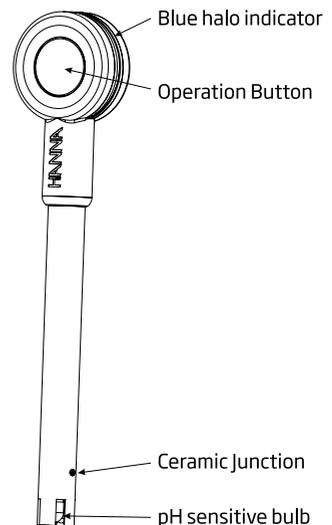
3. Select your probe in the list of visible probes and press **CFM**. The blue LED will start flashing 4 times a second while connecting, then it will slow down and flash every 2 seconds showing it is connected and ready to measure.
