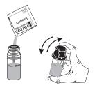
Insert the cuvette into the holder and ensure that the notch on the cap is positioned securely in the groove.
