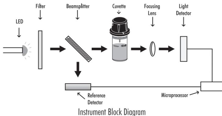
The internal reference system (reference detector) of the [HI97710](#) photometer compensates for any drifts due to power fluctuations or ambient temperature changes, providing a stable source of light for your blank (zero) measurement and sample measurement.
