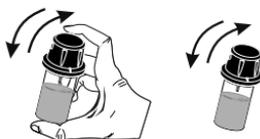
In order to avoid reagent leaking and to obtain more accurate measurements, close the cuvette first with the supplied HDPE plastic stopper
