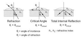
In the HI96803, light from an LED passes through a prism in contact with the sample. An image sensor determines the critical angle at which the light is no longer refracted through the sample. The HI96803 automatically applies temperature compensation to the measurement and converts the refractive index of the sample to Glucose concentration in units of percent (by weight).
