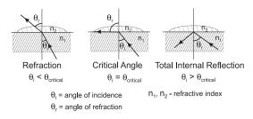
In the H196802, light from an LED passes through a prism in contact with the sample. An image sensor determines the critical angle at which the light is no longer refracted through the sample. The H196802 automatically applies temperature compensation to the measurement and converts the refractive index of the sample to Fructose concentration in units of percent (by weight).
