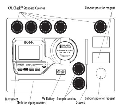
The HI96725 is an auto diagnostic portable microprocessor meter that benefits from Hanna Instruments' years of experience as a manufacturer of analytical instruments. It has an advanced optical system based on a special tungsten lamp and a narrow band interference filter that allows most accurate and repeatable readings. All instruments are factory calibrated and the electronic and optical design minimizes the need of frequent calibration.
