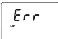
**Cap error:** Appears when external light enters in the analysis cell. Assure that the cuvette cap is present.
