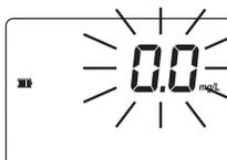
**Under range:** A blinking "0" indicates that the sample absorbs less light than the zero reference. Check the procedure and make sure you use the same cuvette for reference (zero) and measurement.
