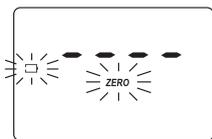
**Battery low:** The battery must be replaced soon.
