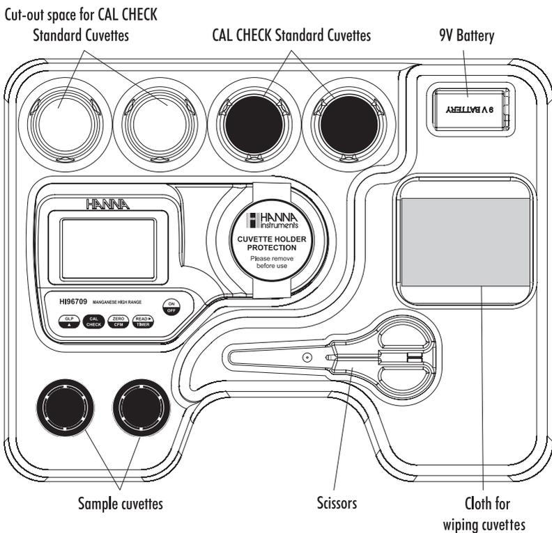
The **HI96709** is an auto diagnostic portable microprocessor meter that benefits from Hanna Instruments' years of experience as a manufacturer of analytical instruments. It has the advanced optical system based on a special tungsten lamp and a narrow band interference filter that allows most accurate and repeatable readings. All instruments are factory calibrated and the electronic and optical design minimizes the need of frequent calibration.
