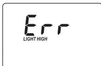
**Light High:** There is too much light to perform a measurement. Please check the preparation of the zero cuvette.
