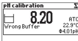
Check if the correct buffer has been used or regenerate the pH electrodes by following the Cleaning Procedure (see ELECTRODE CONDITIONING & MAINTENANCE section). If necessary change the buffer or the electrode.
