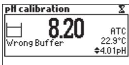
The “Wrong Buffer” message is displayed when the pH value is outside of the acceptable range. Clean the electrode by following the Cleaning Procedure and/or check the buffer concentration before continuing the pH calibration.
