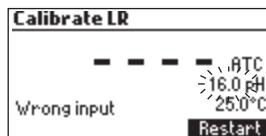
This error message appears when the pH reading exceeds the acceptable input limits ( $-2.00 < \text{pH} < 16.00$ ).
