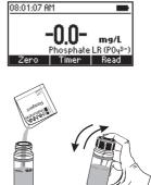
• Insert the cuvette into the holder and close the lid.
