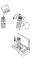
• Press **Timer** and the display will show the countdown prior to the measurement or wait 45 seconds and press **Read**. When the timer ends the meter will perform the reading. The instrument displays the results in **mg/L** of **copper (Cu)**.
