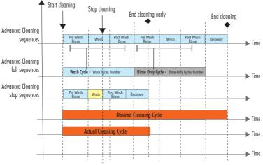
Figure 55: End Cleaning, Stop Sequences
