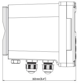
Figure 6: HI520 Controller Fastened to Wall-Mount Panel
