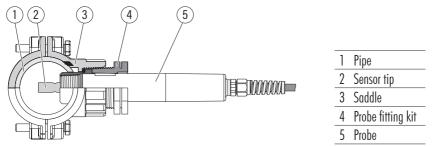
**Note:** To prevent air entrapment inside the electrode the probe can be rotated and horizontal mounting is the recommended option.
