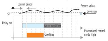
Figure 34: Proportional Control, Relay Out - Proportional Control Mode High, Overtime
