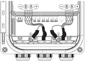
Figure 21: Probes Wiring
