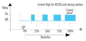
Figure 31: Control High with Relay On, Set Point and Deviation
