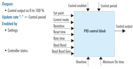
Figure 37: PID Control Block
