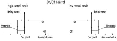
Figure 24: On/Off Control, High /Low Control Mode
