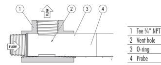
22.2.5. Tank Immersion with Submersible Electrode Holder
