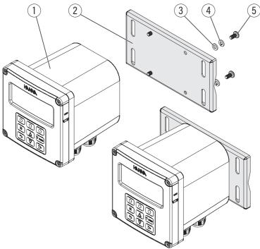
Figure 7: Wall-Mount Schematic
