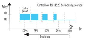
Figure 30: Control Low with Relay On, Set Point and Deviation
