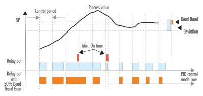
Figure 46: PID Control Mode Low, Relay Out with 50 % Dead Band Gain
