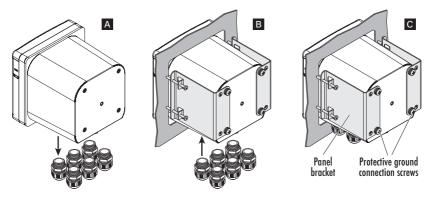
Figure 11: Panel-Mount Steps, Parts (A) (B) (C)
