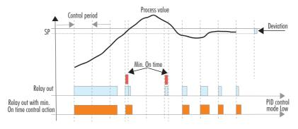
Figure 44: PID Control Mode Low, Relay Out with Minimum On Time
