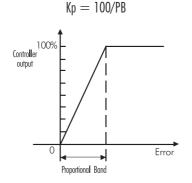
Figure 38: Proportional Action by Means of Proportional Band
