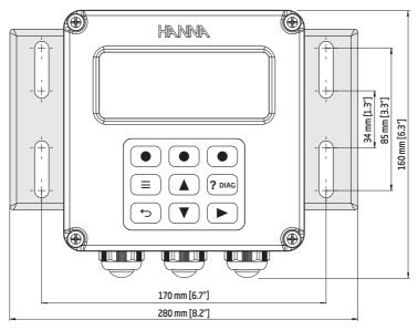
Figure 4: Wall-Mount Panel, Slots Dimensions
