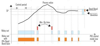
Figure 45: PID Control Mode Low, Relay Out with 0 % Dead Band Gain
