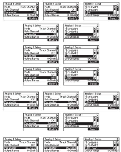
When analog output is assigned to CtrlSetPx, it will follow specific Set point control output.
