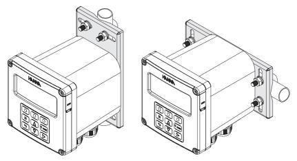
Figure 13: Vertical & Horizontal Pipe Mount
