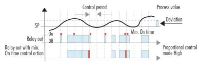
Figure 35: Proportional Control, Relay Out, Proportional Control Mode High, Min. On Time
