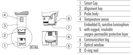
Figure 70: Smart cap detail (HI7640-58 industrial optical DO)
