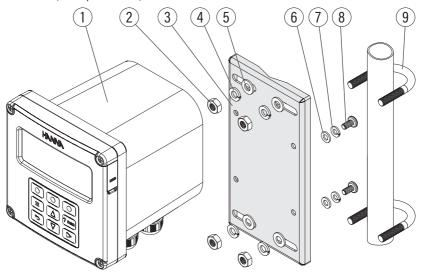
Figure 12: Pipe-Mount Schematic
