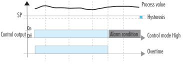
Figure 27: On/Off Control, Overtime Control Action
