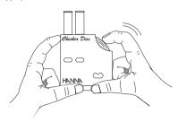
For best results: Perform the reading three times and take the average value (divide by 3 the sum of the three numbers). Intensely colored samples will make the color matching difficult and they should be adequately treated before performing the test. Suspended matter in large amounts should be removed by prior filtration.
