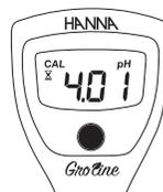
If pH 4 or 10 buffer solution is used as the first point the value of the buffer is recognized and displayed with the blinking stability indicator.
