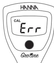
In calibration mode, if the meter displays an "Err" message when in the correct fresh buffer solution then the probe should be cleaned. Place the probe in the HI700501 cleaning solution for 15 minutes. Rinse with purified water and place in storage solution for 1 hour before calibrating. If the "Err" message persists then the HI1271 probe should be replaced.
