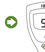
pH 4 will then blink on the display. Press the button to exit and save calibration. "Sto" will then be displayed.
