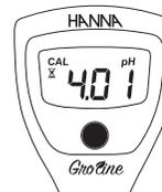
When the reading is stable, the stability indicator will disappear and pH 7 will be calibrated. If pH 7 is the only calibration point, finish one-point procedure at right.
