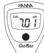
When "7.01" blinks on the display, place the tip of the probe into a pH 4, 7, or 10 buffer solution.
