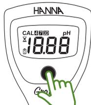
Press the ON/OFF button to turn the meter on. All tags will be displayed.
