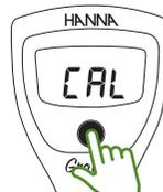
From measurement mode, press and hold the ON/OFF button until "CAL" is displayed.
