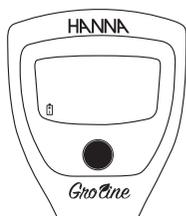
The HI98115 features a low battery indicator. When the battery is running low, the tag will blink on screen. When the battery has been depleted, "Err" will appear on screen and the meter will turn off.
