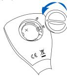
To change the CR2032 Li-ion battery, turn the battery cover located on the back of the meter counterclockwise to unlock. Remove cover and replace with + side facina up.
