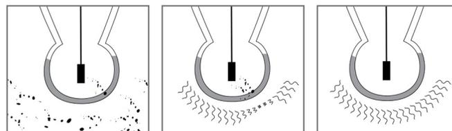
Over time, particles during routine measurement can contaminate the sensor tip.
