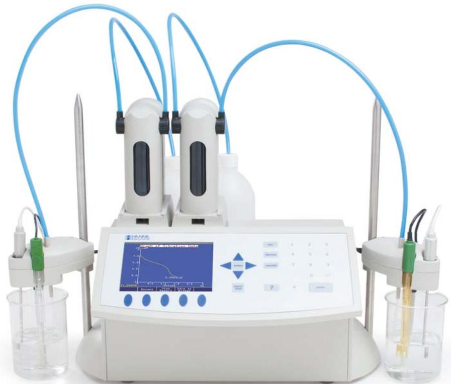
**Standard potentiometric titrator that can measure titratable acidity, sulfur dioxide, yeast assimilable nitrogen (YAN), and reducing sugars.**
