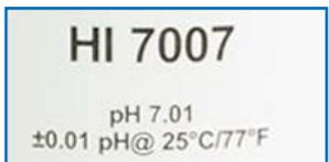
pH calibration buffers should have reported values that are accurate to +/- 0.01 pH @ 25°C and are traceable to NIST Standard Reference Materials.
