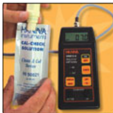
Immerse the probe in HI 50021 check solution
